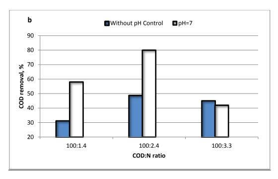
Fig. 6: Effects of COD:N ratio and pH on (a) glucose conversion and (b) COD removal at a COD loading rate of 40 kgm<sup>-3</sup> d<sup>-1</sup>, ambient temperature, and 24 h HRT.
