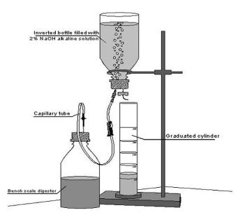
Fig 3: Experimental equipment used to measure the daily methane production.
