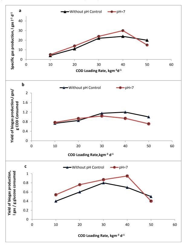
Fig. 5: Effects of COD loading rate and pH on (a) specific production rate,
