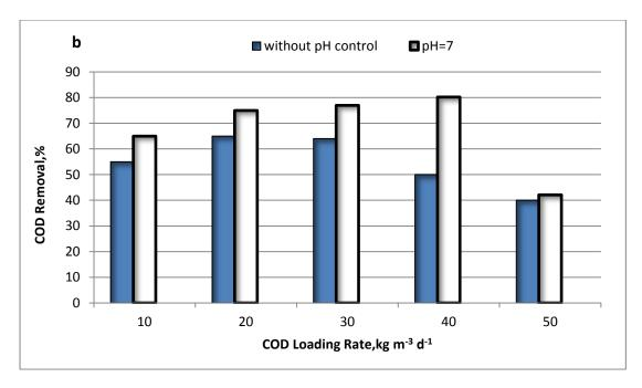
Fig. 4. Effects of COD loading rate and pH on (a) glucose conversion and (b) COD removal at ambient temperature and 24 h HRT.
