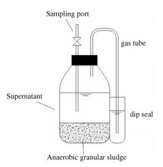
Fig 2: Schematic diagram of anaerobic serum bottle reactor
